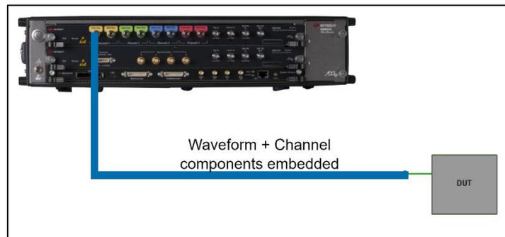
Figure 2: Simplified test setup, with the channel components a part of the generated waveform
