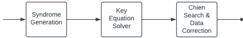
Figure 7. Block diagram of a Reed Solomon code decoder
