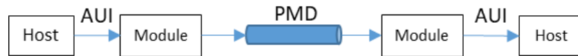
Figure 5. An example of a three-part link containing electrical (AUI) and optical (PMD) sections
