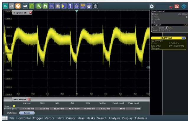
Measurement of a 1.5 V power rail using an R&S®RT-ZP10 10:1, 500 MHz passive probe (50 mV ( V_{pp} ), noise masks signal detail).
