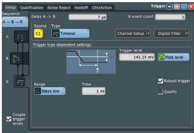
B trigger setup up for the end of the pulse
