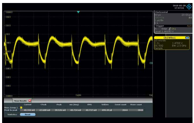
Measurement of a 1.5 V power rail using an R&S®RT-ZPR20 1:1 active power rail probe (~38.3 mV ( V_{pp} )). The captured waveform includes higher frequency transients riding on the rail.
